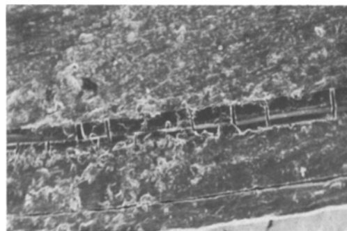
Figure 2 Multiple cracking in boron fibre after 1500 cycles, \times 50 (subsequently reduced by 30% for reproduction).
